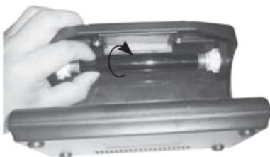
2. To tate the lamp to the place where the lamp pin corresponding to the lamp holder.
